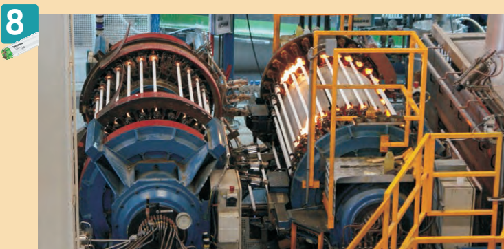
7 The sealing machine then melts the stems to the tubes in which the filaments are mounted
