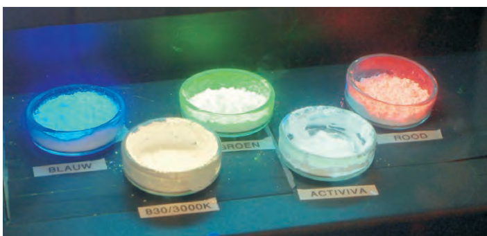
A selection of the different fluorescent powders that can be applied to the phosphor coating
