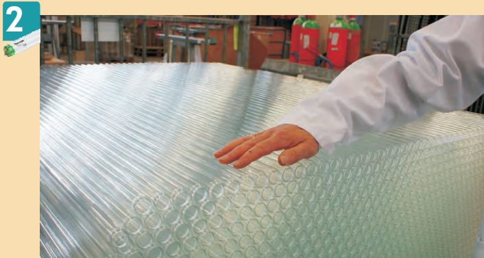
2 Unpacked, the tubes await the first step in their transformation. The 'shoulder' is visible on each tube
