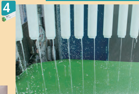
3 Once loaded, the tubes are first washed with demineralised water and then coated with the fluorescent phosphor powder applied as a water suspension
